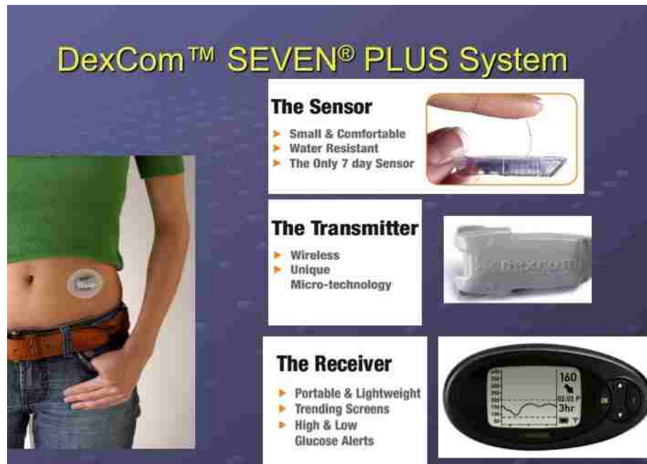
Figure 8. Dexcom SEVEN PLUS™ system. This figure represents the three primary components of the Dexcom SEVEN PLUS™ system.
